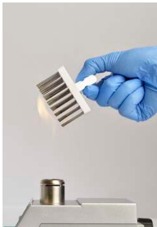
Step 1: Sterilisation using gas burner
