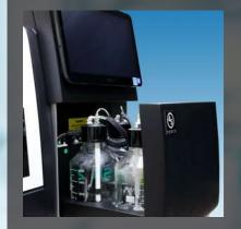
Separate built/in compartment for compressor and hydraulic system.
